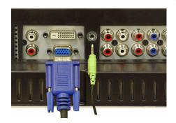
A standard graphic display system for computers that uses an analog signal and can support resolutions up to 1280 x 768.
